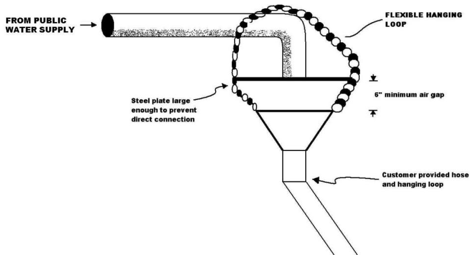
FIGURE 1 – SUGGESTED FILLING DEVICE FOR WATER LOADING STATIONS
