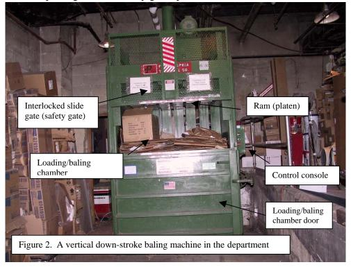
An OSHA compliance officer observed a broken key in the baler's "On or Off" key switch on the day of the incident. A post-incident baler examination found that the electrical wiring had been altered to bypass the "On or Off" switch, and the gate safety switch had been short-circuited by a piece of two-inch wire. By doing so, power was always supplied to the machine and the baler could operate with
