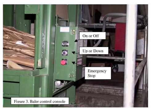
the safety gate up. It could not be determined during this evaluation who modified the baler's electrical circuit, when these alterations were made, and what the intent was.
