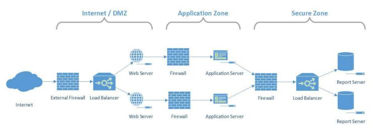
There are several models available for encryption in this architecture. In the first, all traffic in and out of the DMZ is required to be encrypted SSL traffic on port 443. Decryption occurs at the externally facing load balancer and all internal traffic proceeds on unencrypted port 80 communications. This is the most common method used by states and offers both security and optimal performance. This approach is depicted below:
