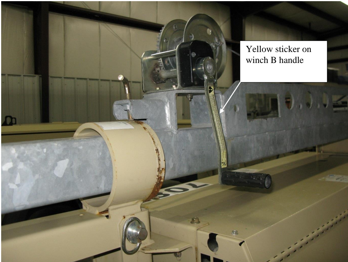
Photo 4. The yellow sticker on winch handles stated that “to raise load, turn handle clockwise” and “to lower load, turn handle counter-clockwise”.
