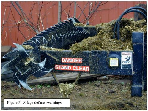
workers including offering worker-training programs. For this particular defacer unit, it was reportedly stressed that the unit should only be energized when the operator was on the tractor and the tractor was in position; otherwise the unit should not be on. It had not been previously observed that any of the workers, including the victim, had ever energized the defacer unit when the tractor was not in position in the bunker silo.
